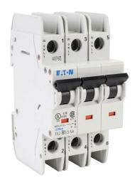
Eaton miniature circuit breaker, current-limiting, 1A, 480Y / 277 VAC / 96 VDC, 3-pole, B curve, thermal magnetic, 10kA @ 480Y/277 VAC interrupting rating, 35mm DIN rail mount.
