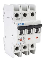
Eaton miniature circuit breaker, current-limiting, 1A, 240 VAC / 96 VDC, 3-pole, B curve, thermal magnetic, 10kA @ 240 VAC interrupting rating, 35mm DIN rail mount.
