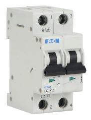
Eaton miniature supplementary protector, 1A, 480Y / 277 VAC / 96 VDC, 2-pole, B curve, thermal magnetic, 10kA @ 480Y/277 VAC interrupting rating, 35mm DIN rail mount.
