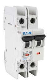
Eaton miniature circuit breaker, current-limiting, 1A, 480Y / 277 VAC / 96 VDC, 2-pole, B curve, thermal magnetic, 10kA @ 480Y/277 VAC interrupting rating, 35mm DIN rail mount.
