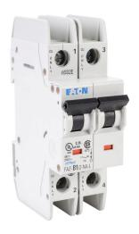
Eaton miniature circuit breaker, current-limiting, 1A, 240 VAC / 96 VDC, 2-pole, B curve, thermal magnetic, 10kA @ 240 VAC interrupting rating, 35mm DIN rail mount.
