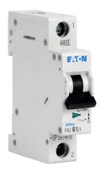
Eaton miniature supplementary protector, 1A, 277 VAC / 48 VDC, 1-pole, B curve, thermal magnetic, 10kA @ 277 VAC interrupting rating, 35mm DIN rail mount.
