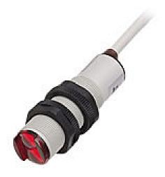
AutomationDirect photoelectric sensor, tubular, threaded, plastic, diffuse with background suppression, 30-130mm sensing distance, complementary light-on/dark-on, NPN, potentiometer, 1 kHz switching frequency, 6.5ft/2m cable length, pigtail.
