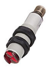
AutomationDirect photoelectric sensor, tubular, threaded, plastic, diffuse with background suppression, 30-130mm sensing distance, selectable light-on/dark-on, PNP, potentiometer, 1 kHz switching frequency, 4-pin M12 quick-disconnect.
