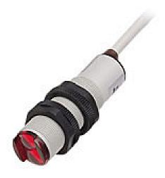
AutomationDirect photoelectric sensor, tubular, threaded, plastic, diffuse with background suppression, 30-130mm sensing distance, selectable light-on/dark-on, PNP, potentiometer, 1 kHz switching frequency, 6.5ft/2m cable length, pigtail.
