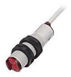
AutomationDirect photoelectric sensor, tubular, threaded, plastic, diffuse with background suppression, 30-130mm sensing distance, selectable light-on/dark-on, NPN, potentiometer, 1 kHz switching frequency, 6.5ft/2m cable length, pigtail.
