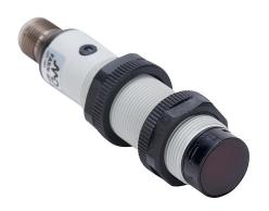
AutomationDirect photoelectric sensor, tubular, threaded, polarized retroreflective, visible red light emission, 3m sensing distance, complementary light-on/dark-on, PNP, potentiometer, 4-wire, 4-pin M12 quick-disconnect.
