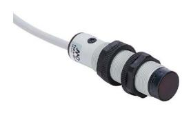
AutomationDirect photoelectric sensor, tubular, threaded, polarized retroreflective, visible red light emission, 3m sensing distance, complementary light-on/dark-on, PNP, potentiometer, 4-wire, pigtail.
