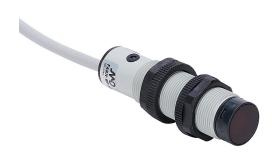
AutomationDirect photoelectric sensor, tubular, threaded, polarized retroreflective, visible red light emission, 3m sensing distance, complementary light-on/dark-on, PNP, potentiometer, 4-wire, pigtail.
