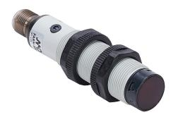
AutomationDirect photoelectric sensor, tubular, threaded, polarized retroreflective, visible red light emission, 3m sensing distance, complementary light-on/dark-on, NPN, potentiometer, 4-wire, 4-pin M12 quick-disconnect.
