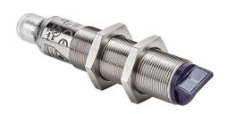
AutomationDirect photoelectric sensor, tubular, threaded, nickel-plated brass, diffuse with background suppression, 90-degree, 30-80mm sensing distance, complementary light-on/dark-on, NPN, potentiometer, 1.5 kHz switching frequency, 4-pin M12 quick-disconnect.
