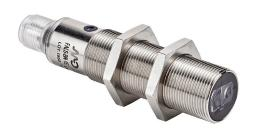
AutomationDirect photoelectric sensor, tubular, threaded, nickelplated brass, diffuse with background suppression, 30-100mm sensing distance, complementary light-on/dark-on, NPN, potentiometer, 1.5 kHz switching frequency, 4-pin M12 quickdisconnect.
