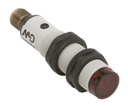
AutomationDirect photoelectric sensor, tubular, threaded, polarized retroreflective, Class 1 laser light emission, 0.06-30m sensing distance, complementary light-on/dark-on, PNP, potentiometer, 4-wire, 4-pin M12 quick-disconnect.
