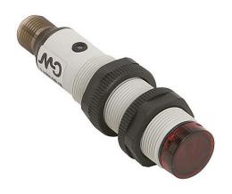
AutomationDirect photoelectric sensor, tubular, threaded, polarized retroreflective, Class 1 red laser, 0.06-30m sensing distance, complementary light-on/dark-on, PNP, potentiometer, 4-wire, 4-pin M12 quick-disconnect.
