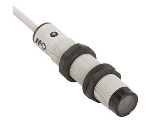
AutomationDirect photoelectric sensor, tubular, threaded, polarized retroreflective, Class 1 laser light emission, 0.06-30m sensing distance, complementary light-on/dark-on, PNP, potentiometer, 4-wire, pigtail.
