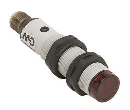
AutomationDirect photoelectric sensor, tubular, threaded, polarized retroreflective, Class 1 red laser, 0.06-30m sensing distance, complementary light-on/dark-on, NPN, potentiometer, 4-wire, 4-pin M12 quick-disconnect.
