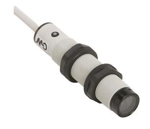
AutomationDirect photoelectric sensor, tubular, threaded, polarized retroreflective, Class 1 red laser, 0.06-30m sensing distance, complementary light-on/dark-on, NPN, potentiometer, 4-wire, pigtail.
