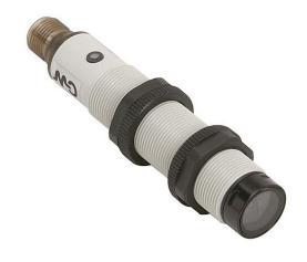
AutomationDirect photoelectric sensor, tubular, threaded, plastic housing, through-beam emitter, Class 1 red laser, 50m sensing distance, 10-30 VDC operating voltage, 2-wire, 4-pin M12 quick-disconnect.
