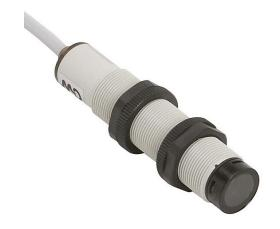
AutomationDirect photoelectric sensor, tubular, threaded, plastic housing, through-beam emitter, Class 1 red laser, 50m sensing distance, 10-30 VDC operating voltage, 2-wire, pigtail.
