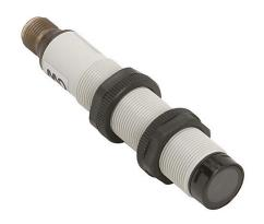
AutomationDirect photoelectric sensor, tubular, threaded, plastic housing, through-beam receiver, 0.1-50m sensing distance, 10-30 VDC operating voltage, complementary light-on/dark-on, PNP, 4-wire, 4-pin M12 quick-disconnect.
