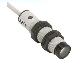
AutomationDirect photoelectric sensor, tubular, threaded, plastic housing, through-beam receiver, 0.1-50m sensing distance, 10-30 VDC operating voltage, complementary light-on/dark-on, PNP, 4-wire, pigtail.
