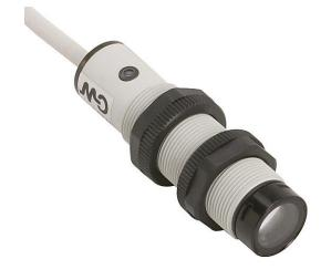
AutomationDirect photoelectric sensor, tubular, threaded, plastic housing, through-beam receiver, 0.1-50m sensing distance, 10-30 VDC operating voltage, complementary light-on/dark-on, PNP, 4-wire, pigtail.
