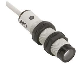
AutomationDirect photoelectric sensor, tubular, threaded, plastic housing, through-beam receiver, 0.1-50m sensing distance, 10-30 VDC operating voltage, complementary light-on/dark-on, NPN, 4-wire, pigtail.
