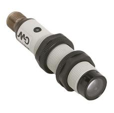
AutomationDirect photoelectric sensor, tubular, threaded, diffuse, Class 1 red laser, 10-300mm sensing distance, complementary light-on/dark-on, PNP, potentiometer, 800 Hz switching frequency, plastic housing, 4-pin M12 quick-disconnect.
