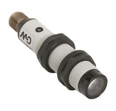
AutomationDirect photoelectric sensor, tubular, threaded, diffuse, Class 1 laser light emission, 10-300mm sensing distance, complementary light-on/dark-on, PNP, potentiometer, 800 Hz switching frequency, plastic housing, 4-pin M12 quick-disconnect.
