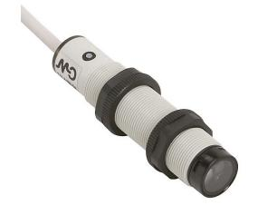
AutomationDirect photoelectric sensor, tubular, threaded, diffuse, Class 1 red laser, 10-300mm sensing distance, complementary light-on/dark-on, PNP, potentiometer, 800 Hz switching frequency, plastic housing, pigtail.
