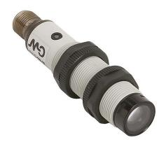
AutomationDirect photoelectric sensor, tubular, threaded, diffuse, Class 1 laser light emission, 10-300mm sensing distance, complementary light-on/dark-on, NPN, potentiometer, 800 Hz switching frequency, plastic housing, 4-pin M12 quick-disconnect.
