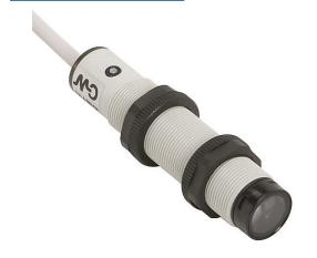
AutomationDirect photoelectric sensor, tubular, threaded, diffuse, Class 1 red laser, 10-300mm sensing distance, complementary light-on/dark-on, NPN, potentiometer, 800 Hz switching frequency, plastic housing, pigtail.
