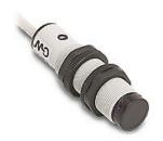
AutomationDirect photoelectric sensor, tubular, threaded, plastic housing, through-beam emitter, 20m sensing distance, 10-30 VDC operating voltage, 2-wire, pigtail.
