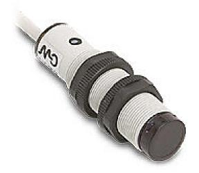
AutomationDirect photoelectric sensor, tubular, threaded, plastic housing, through-beam emitter, infrared light emission, 20m sensing distance, 10-30 VDC operating voltage, 2-wire, pigtail.
