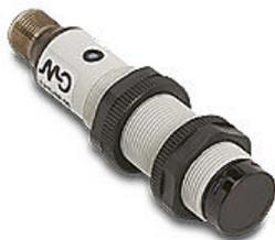
AutomationDirect photoelectric sensor, tubular, threaded, plastic housing, through-beam receiver, 20m sensing distance, 10-30 VDC operating voltage, complementary light-on/dark-on, PNP, 4-wire, 4-pin M12 quick-disconnect.
