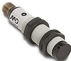
AutomationDirect photoelectric sensor, tubular, threaded, plastic housing, through-beam receiver, 20m sensing distance, 10-30 VDC operating voltage, complementary light-on/dark-on, NPN, 4-wire, 4-pin M12 quick-disconnect.
