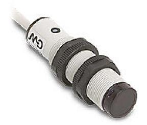
AutomationDirect photoelectric sensor, tubular, threaded, plastic housing, through-beam receiver, 20m sensing distance, 10-30 VDC operating voltage, complementary light-on/dark-on, NPN, 4-wire, pigtail.
