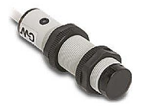
AutomationDirect photoelectric sensor, tubular, threaded, diffuse, infrared light emission, 1m sensing distance, complementary light-on/dark-on, PNP, 250 Hz switching frequency, plastic housing, pigtail.
