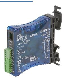
AutomationDirect serial converter, RS-232 (RJ12) to RS-422/485 (5-pin terminal), isolation protection, 5 VDC from PLC or 24 VDC external nominal input, encapsulated, DIN rail or panel mount.
