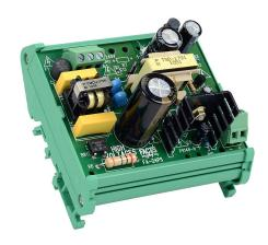
AutomationDirect switching power supply, 24 VDC @ 1.25A/30W, 120/240 VAC nominal input, 1-phase, open frame, plastic housing, 35mm DIN rail mount, screw terminals, hazardous location rated.
