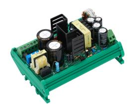
AutomationDirect switching power supply, 24 VDC @ 3.7A/90W, 120/240 VAC nominal input, 1-phase, open frame, plastic housing, 35mm DIN rail mount, screw terminals, hazardous location rated.
