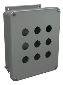
Stahlin F series pushbutton enclosure, 9 holes, 30mm, NEMA 1/3R/4X/6P/12, 11 x 9 x 4in (HxWxD), wall mount, fiberglass reinforced polyester, gray, screw cover, purchase subpanel separately.
