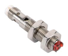
ProSense photoelectric sensor, tubular, threaded, stainless steel, diffuse with background suppression, 7-30mm sensing distance, light-on, PNP, potentiometer, 450 Hz switching frequency, 3-pin M8 quick-disconnect.
