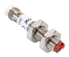
ProSense photoelectric sensor, tubular, threaded, stainless steel, diffuse with background suppression, 0-20mm sensing distance, light-on, PNP, 450 Hz switching frequency, 3-pin M8 quick-disconnect.
