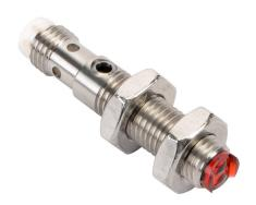
ProSense photoelectric sensor, tubular, threaded, stainless steel, diffuse with background suppression, 7-30mm sensing distance, light-on, NPN, potentiometer, 450 Hz switching frequency, 3-pin M8 quick-disconnect.
