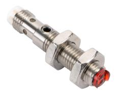
ProSense photoelectric sensor, tubular, threaded, stainless steel, diffuse with background suppression, 7-30mm sensing distance, light-on, NPN, potentiometer, 450 Hz switching frequency, 3-pin M8 quick-disconnect.
