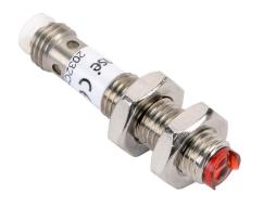
ProSense photoelectric sensor, tubular, threaded, stainless steel, diffuse with background suppression, 0-20mm sensing distance, light-on, NPN, 450 Hz switching frequency, 3-pin M8 quick-disconnect.
