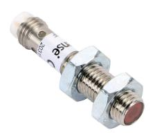
ProSense photoelectric sensor, tubular, threaded, stainless steel housing, through-beam receiver, 0-2.2m sensing distance, 10-30 VDC operating voltage, dark-on, PNP, 3-wire, 3-pin M8 quick-disconnect.
