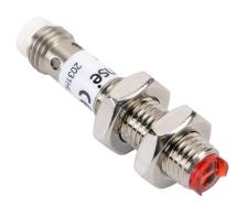
ProSense photoelectric sensor, tubular, threaded, polarized retroreflective, visible red light emission, 0-1m sensing distance, dark-on, PNP, 3-wire, 3-pin M8 quick-disconnect.
