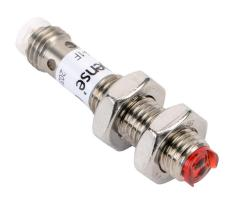
ProSense photoelectric sensor, tubular, threaded, polarized retroreflective, visible red, 0-1m sensing distance, dark-on, NPN, 3-wire, 3-pin M8 quick-disconnect.
