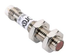
ProSense photoelectric sensor, tubular, threaded, stainless steel housing, through-beam emitter, visible red, 0-2.2m sensing distance, 10-30 VDC operating voltage, 2-wire, 3-pin M8 quick-disconnect.
