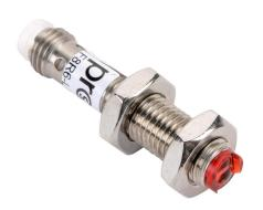
ProSense photoelectric sensor, tubular, threaded, diffuse, visible red, 1-60mm sensing distance, light-on, PNP, 500 Hz switching frequency, stainless steel housing, 3-pin M8 quick-disconnect.
