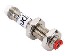
ProSense photoelectric sensor, tubular, threaded, diffuse, visible red light emission, 1-60mm sensing distance, light-on, PNP, 500 Hz switching frequency, stainless steel housing, 3-pin M8 quick-disconnect.
