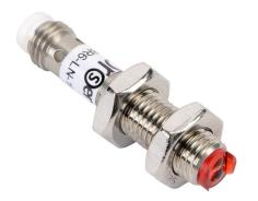
ProSense photoelectric sensor, tubular, threaded, diffuse, visible red, 1-60mm sensing distance, light-on, NPN, 500 Hz switching frequency, stainless steel housing, 3-pin M8 quick-disconnect.
