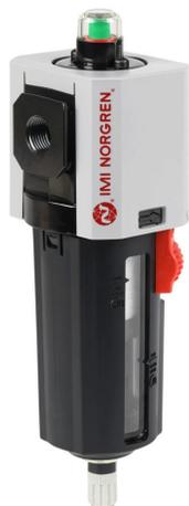
Norgren Excelon Plus 84 pneumatic filter, coalescing oil removal, 3/8in female NPT inlet(s), 3/8in female NPT outlet(s), automatic drain, polycarbonate bowl, bowl guard. For use with Excelon 84 series components.
