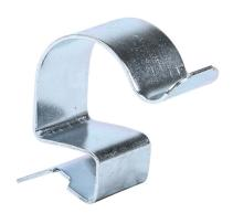
Minerallac flange mount cable clip, package of 100. For use with 3/16 to 9/32in flanges and 0.750-0.937in OD tubing or cable.
