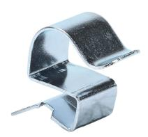
Minerallac flange mount cable clip, package of 100. For use with 3/16 to 9/32in flanges and 0.468-0.562in OD tubing or cable.
